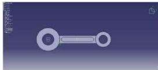
Fig 4 Edge Fillet Sketch (radius =8mm)
